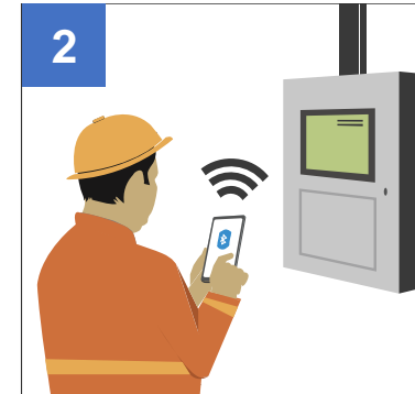
2 Establish a secure Bluetooth connection between mobile app & Fire Alarm Control panel.
